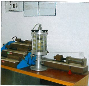
STDTTS型 静三轴及非饱和土试验系统 STDTTS Static Tri-axial and Unsaturated Testing System
